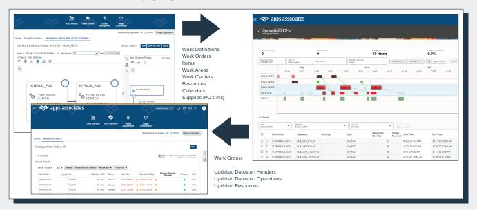
The following is a screen capture from the Oracle Gantt chart displaying a multi-stage manufacturing process where one of three build lines can feed a downstream packing operation.
